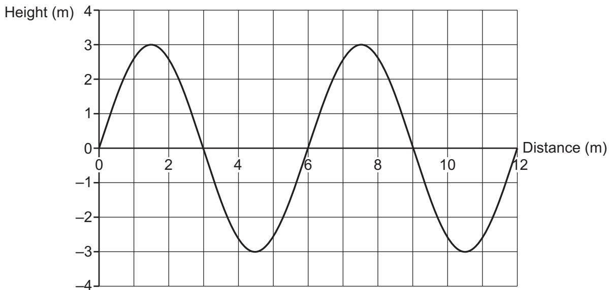
(a) The water wave has a wavelength of 6 m.
