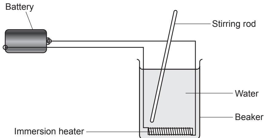
She uses an immersion heater to increase the temperature of the water.
