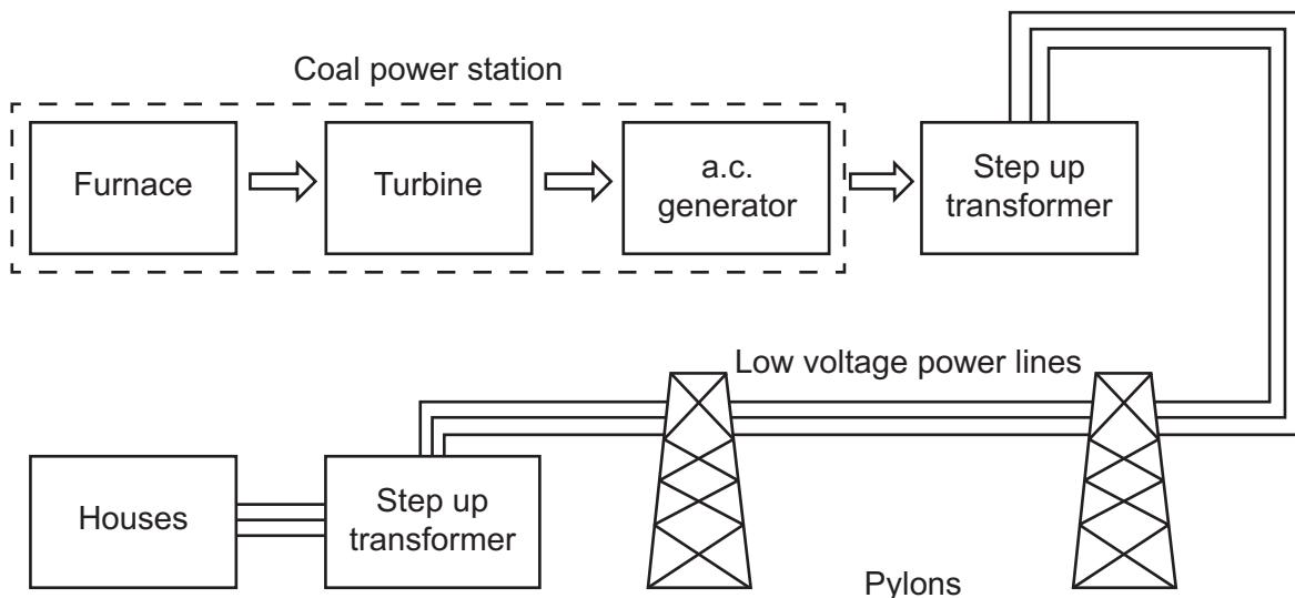
(a) State the **two** mistakes in the diagram.
