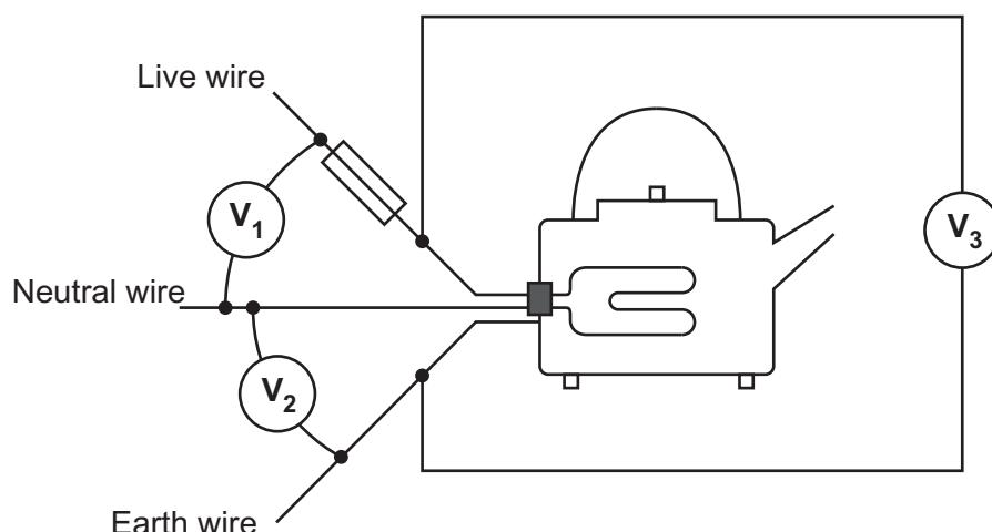
Use the relationship:  $V_3 = V_1 + V_2$
