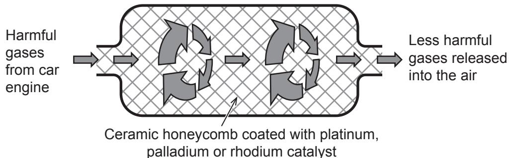
The harmful gases from the car engine do not react with each other until they are in contact with the hot catalyst.
